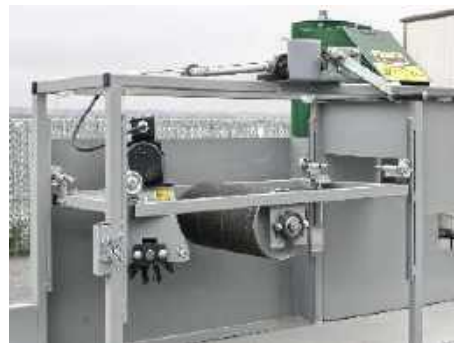
Leveling roller and brush assembly
